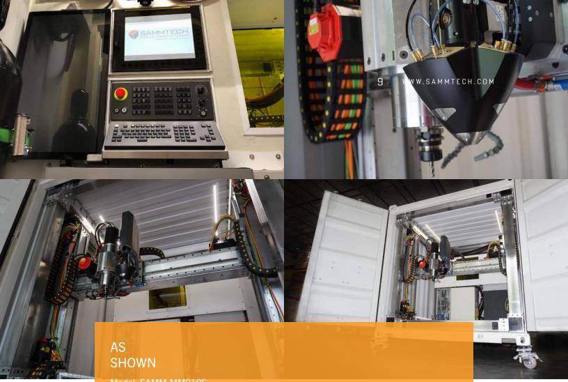
Model: SAMM-MM010S Metal production + milling head built into a 10-ft., standard height shipping container
